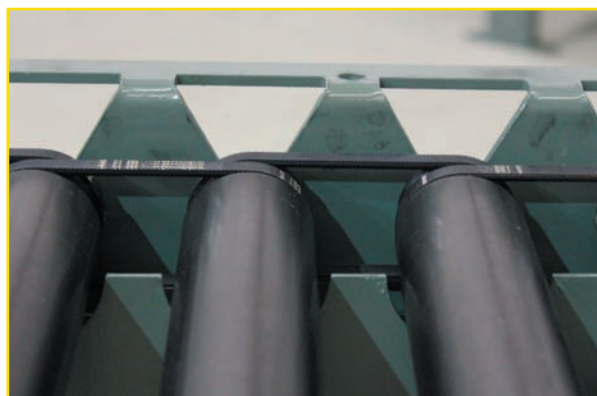
Guard removed to illustrate roll-to-roll drive belt. WARNING: Do not operate conveyor with guard removed.
