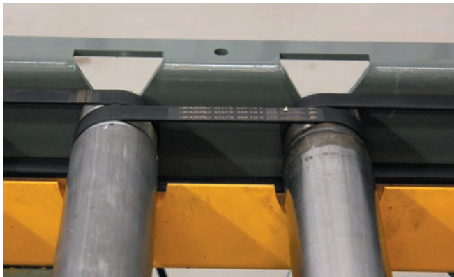
Guard removed to illustrate roll-to-roll drive belt. WARNING: Do not operate conveyor with guard removed.
